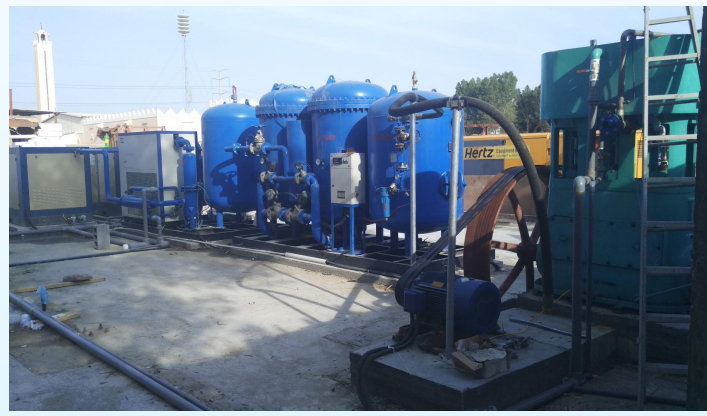
NTK-100P PSA Oxygen Plant - Saudi Arabia
