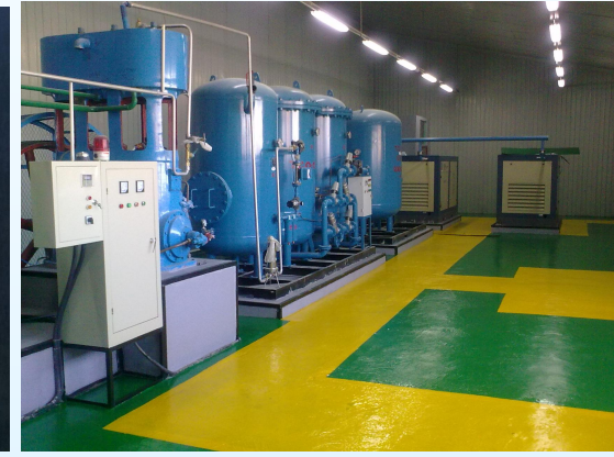
NTK-80P PSA Oxygen Plant - Brazil
